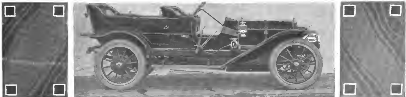
York Motor Car Company Introduces a Toy Tonneau Body for its Four-Cylinder 40-Horsepower Chassis.
